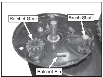
Figure 14. Ratchet gear assembly.
